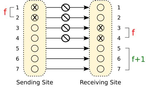
Figure 2: An erasure encoding based logical link is composed of  $3f + 1$  virtual links; in this example,  $f = 2$ . The adversary can block at most  $f$  virtual links by corrupting servers in the sending site and  $f$  virtual links by corrupting servers in the receiving site. Thus, at least  $f + 1$  virtual links have two correct endpoints and can freely pass messages.
