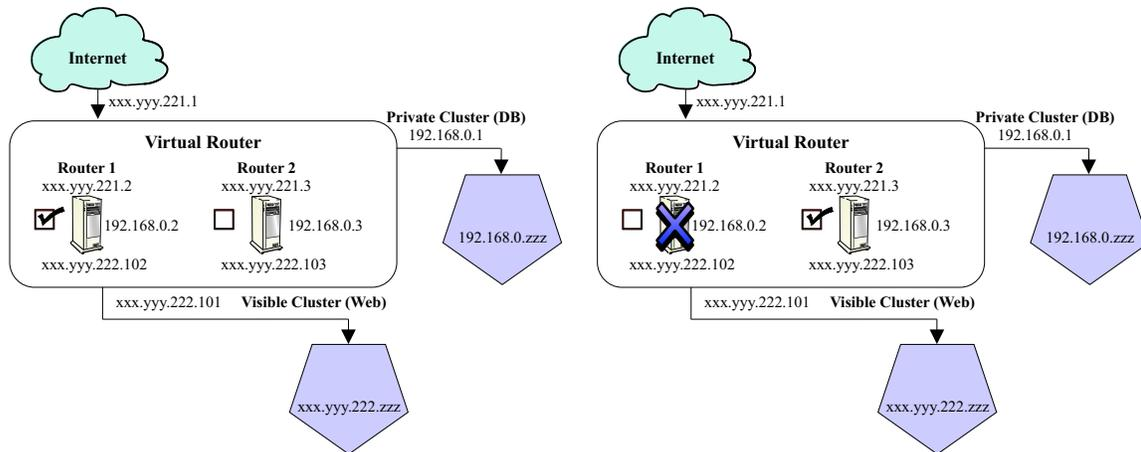
**Figure 4. N-Way Fail-Over for Routers: At any point, a single physical router acts as the virtual router, managing the virtual addresses xxx.yyy.221.1, xxx.yyy.222.101, 192.168.0.1.**
