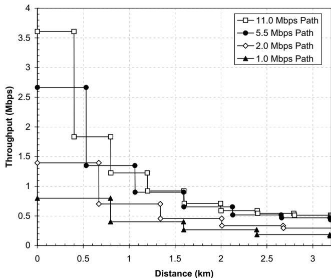
Fig. 6. Throughput Loss Along a Path
