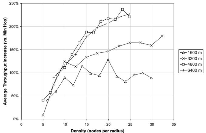
Fig. 10. Average throughput increase of MTM over min hop along a randomized straight line path.
